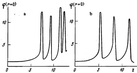
FIG. 3. Field amplitude on the axis (a) for an "undistorted" beam, and (b) for a "distorted" beam.
