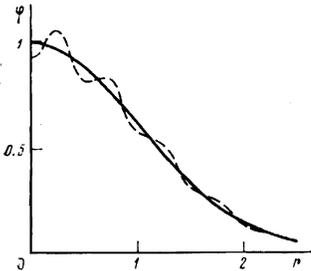
FIG. 4. Initial profiles of the field amplitude: full-drawn line: "undistorted" beam; dashed line: "distorted" beam.
