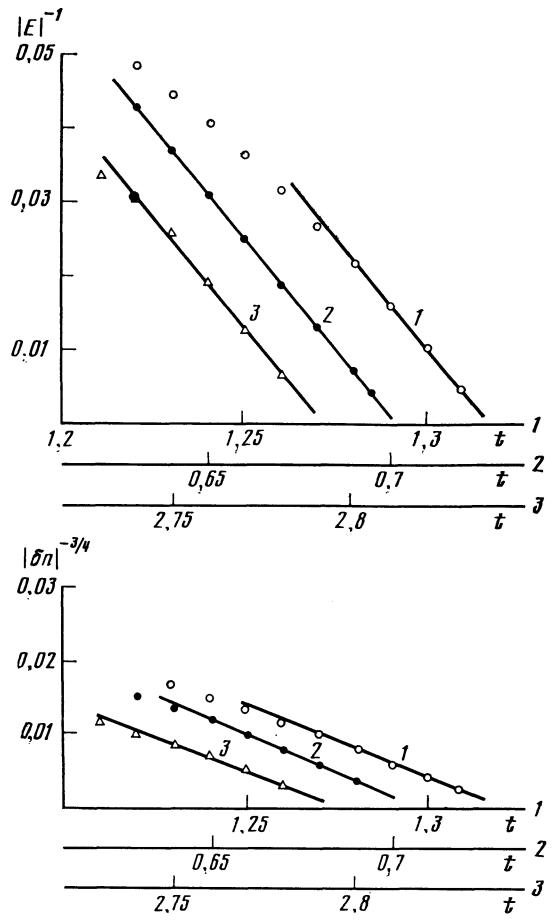
FIG. 2. Self-similar  $t$ -dependence of  $|E|^2$  and  $|\delta n|^{-3/4}$  [the straight lines correspond to Eqs. (8)]: 1) for the variant shown in Fig. 1; 2) for the variant corresponding to the initial conditions (12) in a pumping field  $E_0 = 2.0$ ; 3) for the variant shown in Fig. 3.
