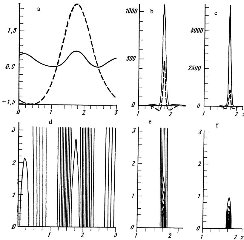
FIG. 3. Dynamics of Langmuir collapse occurring due to the action of a pump  $E_0 = 2.0$  from the initially sinusoidal modulation of field and density in the plasma. a,b,c)  $|E|^2$  (solid curves) and  $-\delta n$  (dashed curves) as functions of  $z$  for  $r = 0$ : a)  $t = 1.45$ , b)  $t = 2.74$ , c)  $t = 2.77$ ; d,e,f) lines of constant  $|E|^2$  at the same times.
