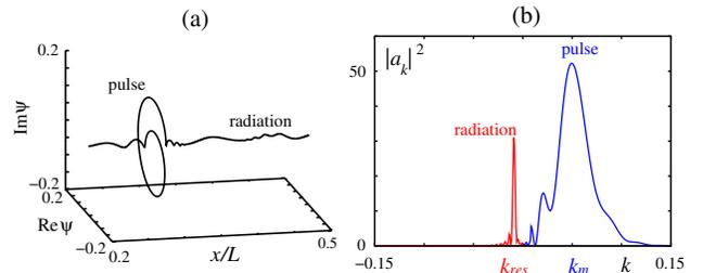
FIG. 4 (color online). (a) Pulse and low-amplitude long wave radiation in space. (b) In Fourier space, the pulse has the maximum power at  $k_m$ . The radiation is a narrow peak at  $k_{\text{res}} \approx -(\sqrt{2} - 1)^2 k_m$ .
