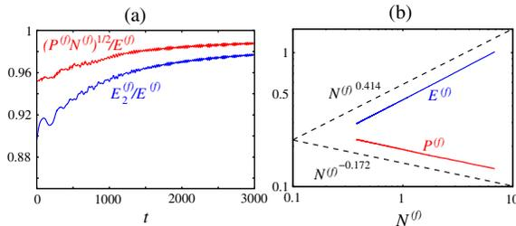
FIG. 5 (color online). (a) The ratios  $(P^{(f)}N^{(f)})^{1/2}/E^{(f)}$  and  $E_2^{(f)}/E^{(f)}$  of an evolving pulse as functions of time. (b) Energy  $E^{(f)} \sim N^{(f)\sqrt{2}-1}$  and the momentum  $P^{(f)} \sim N^{(f)\sqrt{8}-3}$  of an evolving pulse as functions of the wave action  $N^{(f)}$ . The wave action and the energy decrease in time, while the momentum increases.
