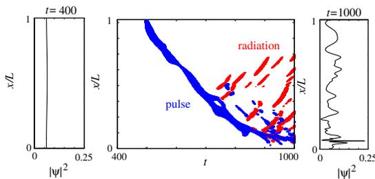
FIG. 3 (color online). Time evolution for the initial condition of  $\psi(x, t = 0) = 0.25 \exp(i2\pi x/L)$  plus weak noise for the MMT equation ( $\lambda = 1$ ) with no damping and driving. The figure shows traces of regions with high momentum density. A pulse appears by the Benjamin-Feir instability of the initial wave. Its speed decays in time as it emits counterpropagating radiation.
