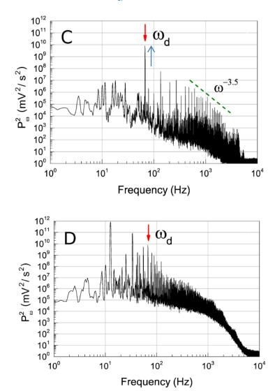
Nonlinear waves at the surface of superfluid He-II in the cylindrical cell of the inner diameter D = 60 mm $w_d = 32\text{Hz}$ ; T = 1.7 K
