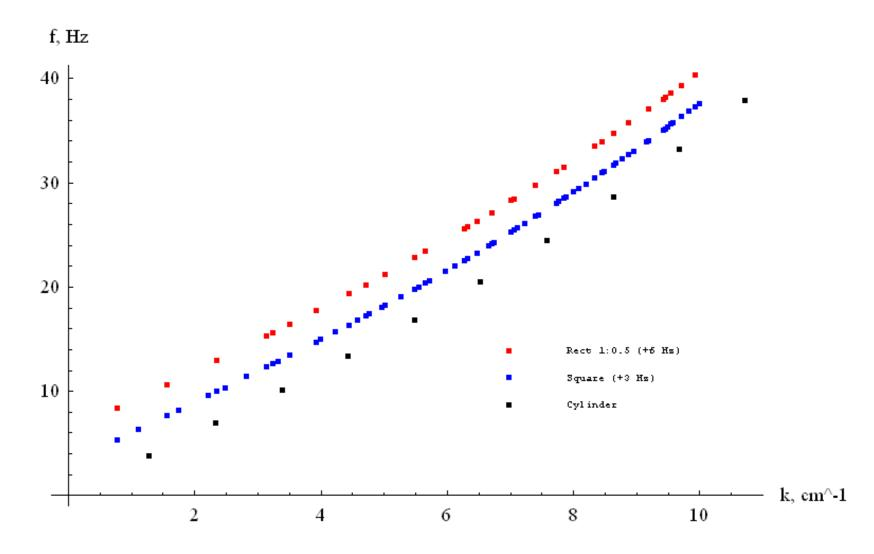
Surface oscillations. The resonant modes in a cell filled with liquid hydrogen: cylinder 6 cm in diameter (dark points • ); a square 3x3 cm (blue points: shifted to 3Hz), and a rectangular channel 4x2 cm in dimensions (red points, shifted to 6 Hz). Number of modes: cylinder – 9 (radial symmetry); square 66; rectangular cell – 50.
