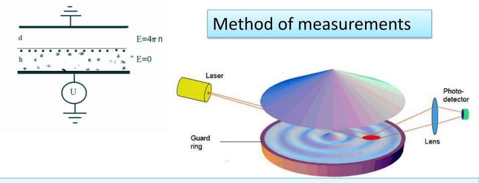
Oscillations of the fluid surface elevation η (r, t) were detected through variations of the power P(t) of the laser beam reflected from the surface. The wave power law
