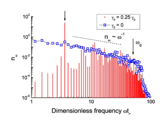
Numerical steady-state spectrum of sustained surface oscillations.
