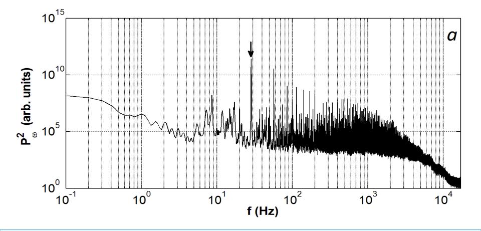
Liquid hydrogen in the rectangular cell with linear dimensions 4.0x2.0 cm; the cell depth h =0.35 cm; the gap between the charged surface and the outer collector d=0.35 cm. The power spectrum P<sub>ω</sub><sup>2</sup>: U<sub>dc</sub> = 800 V, U<sub>p</sub>=220 V, f<sub>p</sub>= ω/2π =28.5 Γц (shown by the arrow).
