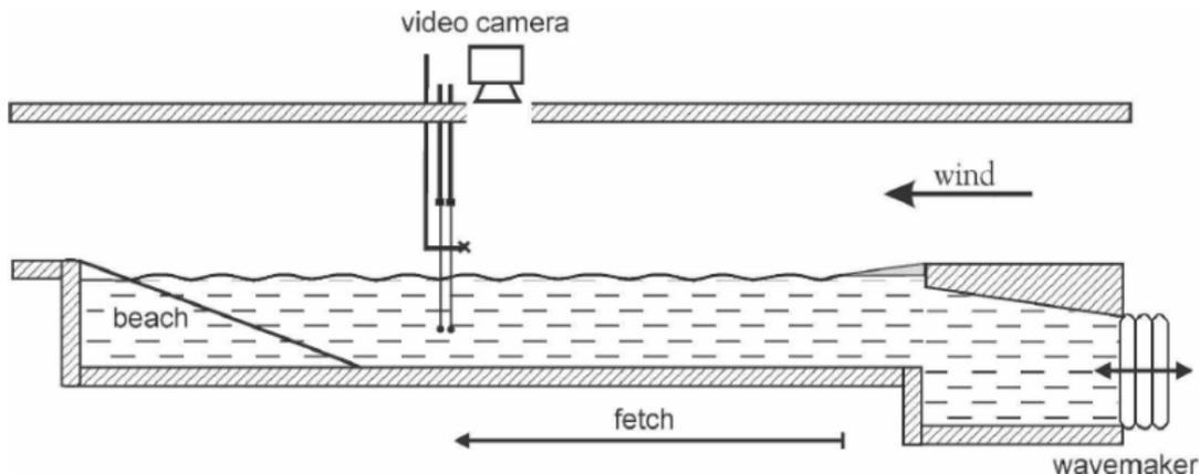
FIG. 1. Schematic view of the large IRPHE-Luminy wind wave tank.
