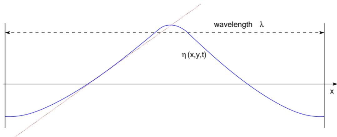
Steepness of the surface  $\mu = \sqrt{\langle |\nabla\eta(\vec{r}, t)|^2 \rangle} \simeq 0.1$  — average slope of the surface.
